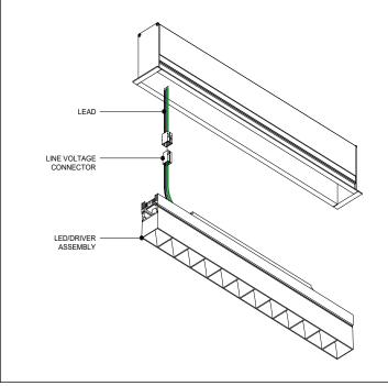
\*\* LED'S SHOULD BE PROTECTED FROM DUST AND DEBRIS DURING INSTALLATION AND MAINTENANCE
