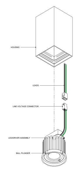
\*\* LED'S SHOULD BE PROTECTED FROM DUST AND DEBRIS DURING INSTALLATION AND MAINTENANCE <u>Click here to read full Care and Maintenance</u>
