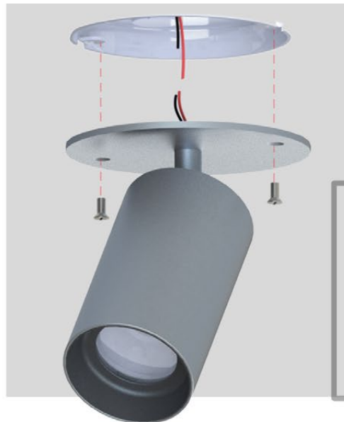
Step 5- Using #8 screws included with canopy, securely fasten canopy plate to pancake box.
