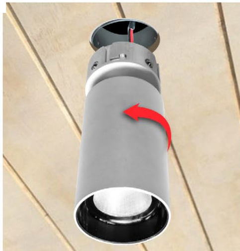
Step 6 and 7- Make sure all electrical components are working prior to inserting fixture in receiver. Align fixture j-hook slots with cleats in receiver. Push up and rotate counter-clockwise until rotation stops and fixture drops to flush position. Canopy should be flush with ceiling. Install complete.
