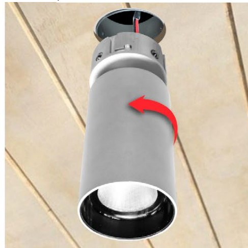
Step 6 and 7- Make sure all electrical components are working prior to inserting fixture in receiver. Align fixture j-hook slots with cleats in receiver. Push up and rotate counter-clockwise until rotation stops and fixture drops to flush position. Canopy should be flush with ceiling. Install complete.
