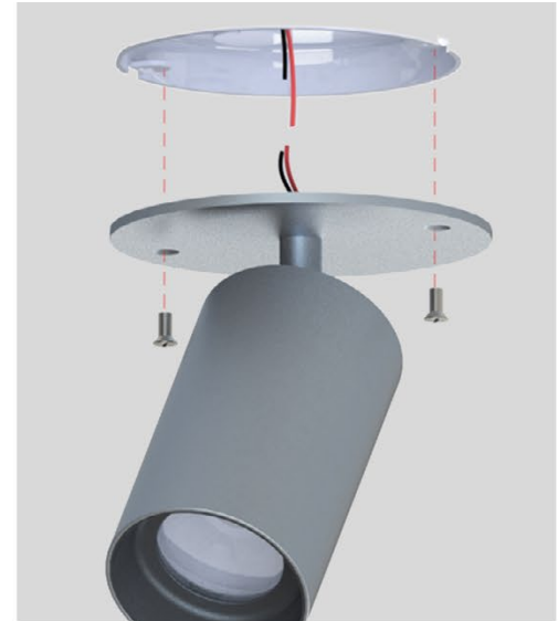
Step 6- Screw canopy plate to pancake box with (2) #8 screws
